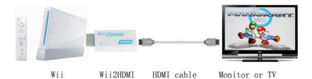
3. Turn on the TV/monitor and switch the video input of the TV to match the HDMI input connector used by the Wii2HDMI. Then you should be able to see the Wii screen after you turn on the Wii console.
